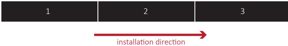
2. Where the first row planks will meet the wall, start by cutting off the tongue from the length of the planks.
